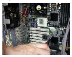
**e.** Take out the Motherboard carefully to avoid any damage.
